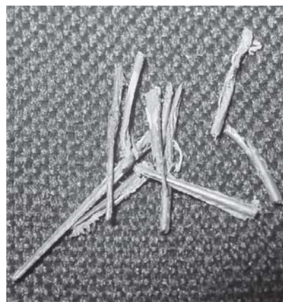
Figure 1 - Carriers cut by instrument friction
