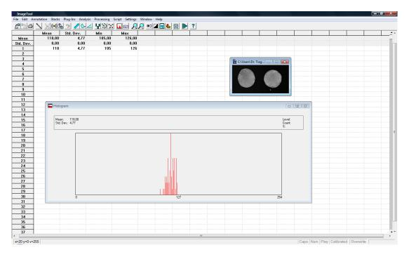
Figure 1 - Radiopacity measurement of the cements through the ImageTool® software
