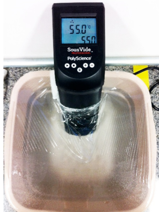
Figure 4 - Thermal cycler (model CRC-5AC2W, PolyScience, Niles, EUA) for the membranes plasticization to keep constant the temperature of saline solution (55°C)
